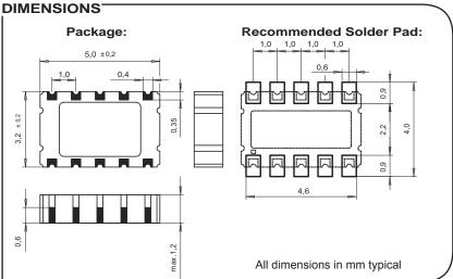
Extremely Accurate RTC Module with embedded Xtal. SPI Interface Temperature Compensation Automotive qualified, according to AEC-Q200 Rev. C
