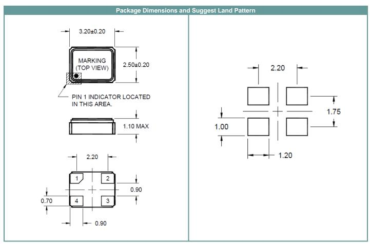
All dimension in millimeters (mm).
