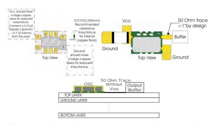
Attention: To achieve optimal frequency stability, and in some cases to meet the specification stated on this data sheet, it is required that the circuit connected to this TCXO output must have the equivalent input capacitance that is specified by the nominal load capacitance. Deviations from the nominal load capacitance will have a graduated effect on the stability of approximately 20 ppb per pF load difference.
