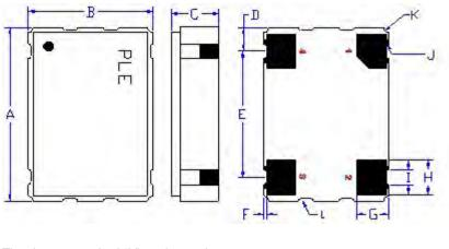
The detents marked "L" on the package ends are optional
