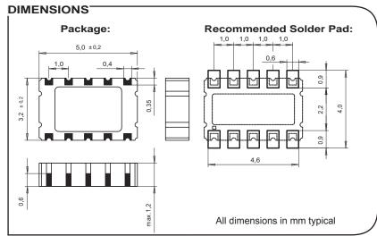
Extremely Accurate RTC Module with embedded Xtal. I<sup>2</sup>C Interface Temperature Compensation Automotive qualified, according to AEC-Q200 Rev. C
