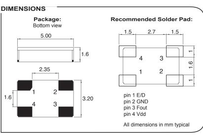
SMT Clock oscillator in ceramic package Fundamental quartz mode frequency High shock and vibration resistance Wide temperature range Low aging Ultra low internal MSL Very fast start-up Excellent solderability Swiss made quality Customer specification on request
